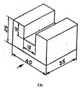
10 Draw the isometric projection of the object from the views shown in figure below. All (14M) dimensions are in mm.
